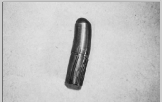
Even monometal bullets are not perfect. This bent specimen is a 300 grain .375 monometal recovered from an elephant carcass.
