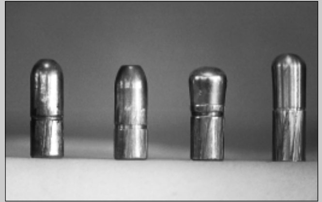
Recovered bullets (L - R): Woodleigh, Speer, A-Square and Barnes. Note flattened tip of the lighter A-Square, although penetration was not affected. Also note slight bend on the Barnes bullet.
